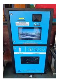
Supply and Installation of automatic branded Plastic bottle crusher machine with capacity of 30 bottle/minute, Material: Plastic bottle crusher machine shall be made of Mild steel, electric motor power: 2 HP, Current: 6 Amperes, Warranty: 5 Years. Plastic bottle crusher machine as approved by engineer In-charge/employer.
